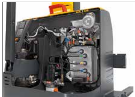
Sealed AC motor, controllers and connectors
